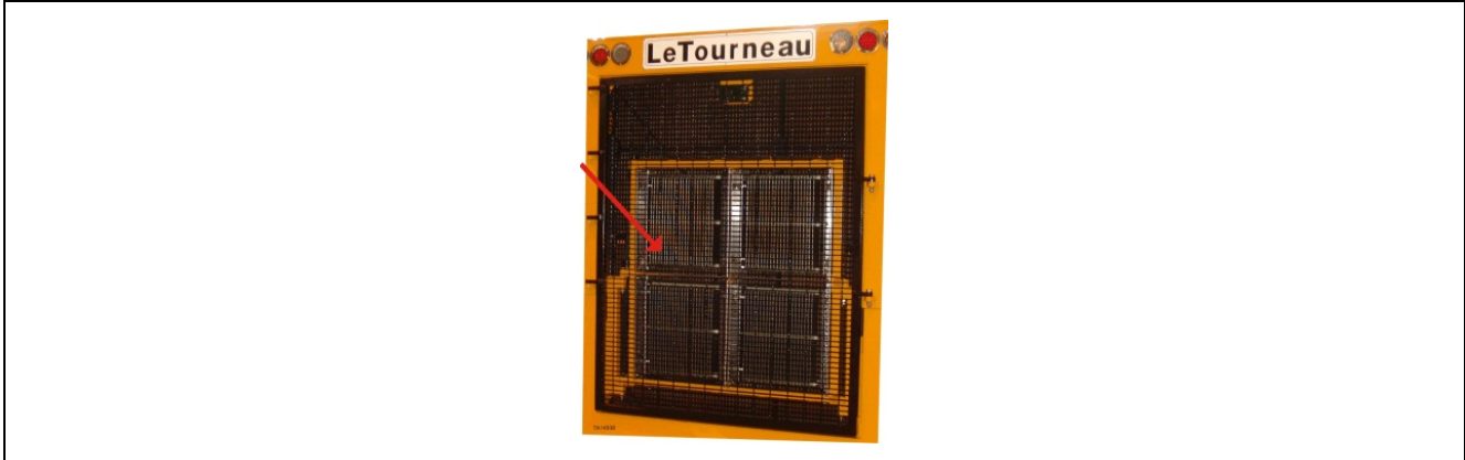
Figure 2. Shock hazards braking grids
