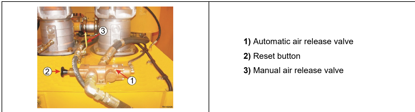
Figure 3. Hydraulic reservoir air release valves
